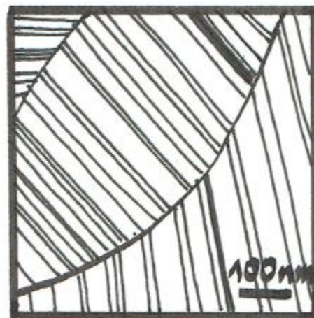
Figure 8: Micrograph showing three ultrafine grains in copper with dense twin boundaries (after [22])
