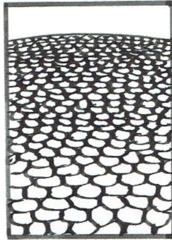
Figure 5: Gradient nano-grained structure in copper (after [18])
