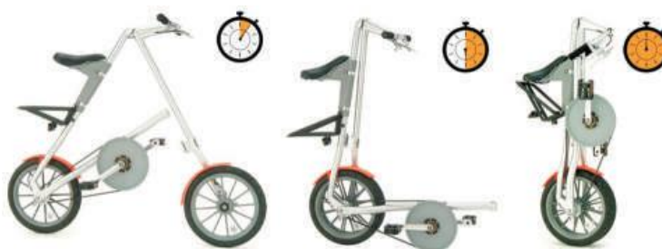
Fig. 3. Other modes (Strida folding Mode)
