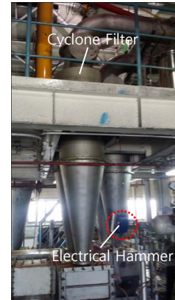
Fig. 4. Cyclone for separation Toner
