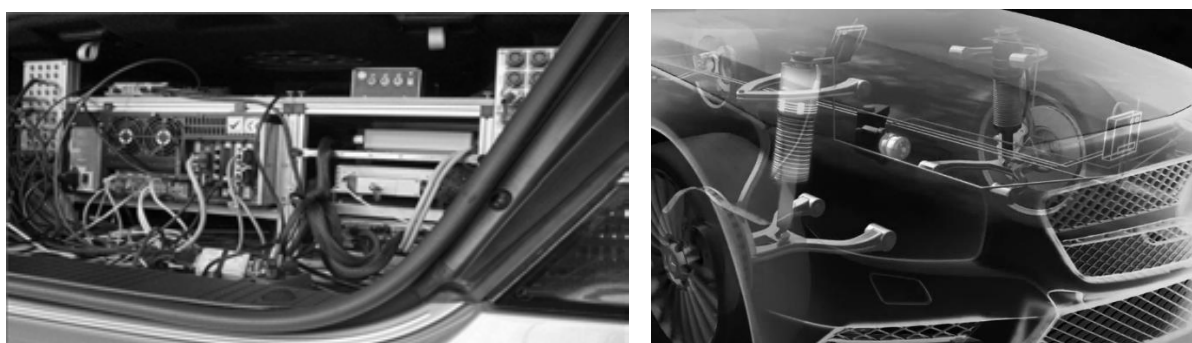
Fig.6 a) Magic Body Control system and b) Active Body Control system
