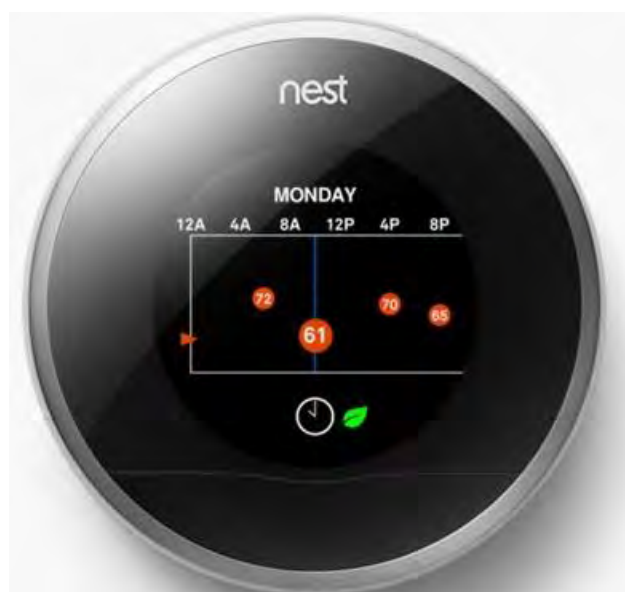
Fig. 1. Nest smart thermostat learns how users set their heating manually, uses motion and light sensor to detect when occupants are at home, and then uses this data to optimize heating schedule and settings
