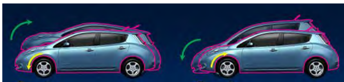
Fig.10 a) torque increase causes raising up the front of the vehicle, b) by torque decrease the front of the vehicle will be lower
