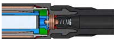
Fig. 6. Improved design with no o-ring.
