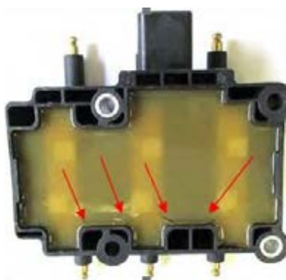
Fig. 1. 6P Ignition coil with cracks after the temperature shock tests
