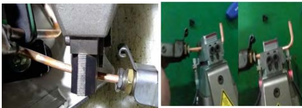
Fig. 6. Equipment condition when tube is not probably touched with blade (left picture) and when tube is well in touch with metal detecting sensor (right picture)
