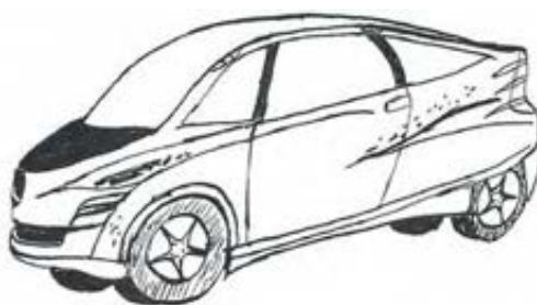
Fig. 2. Mercedes biomimetic concept vehicle based on the female yellow boxfish [22]
