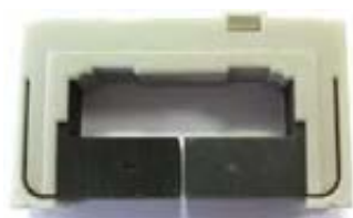
Fig. 2. Plastic covers securing the metal lamination
