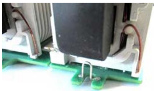
Fig. 4. New spring terminal
